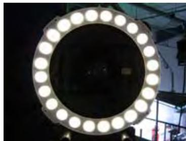
Fluorescents don't have much place as effects lights and probably never will. Don't expect a fluorescent source four ellipsoidal. However with the introduction of an asymmetric reflector and brighter fixtures, they can make great cyc lights.
